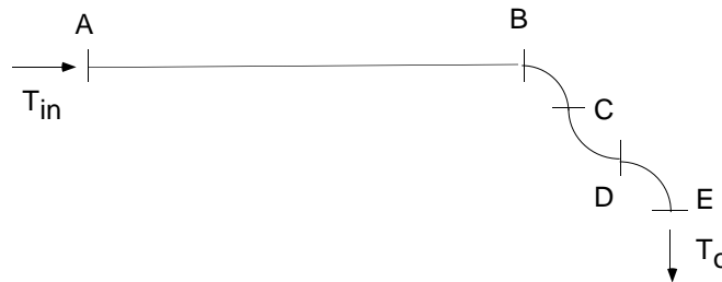
Figure B.1—Conduit layout—Chart development
