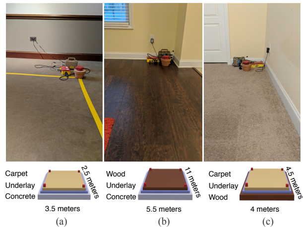
Fig. 10: The three structural types and the sensors configuration for each of them.
