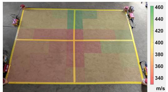
Fig. 5: Floor velocity model initialized by hammer tests.
