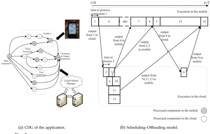
Fig. 2: Scheduling model for cloud offloading in a 14-component mobile application with a general CDG.
