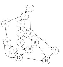
(c) Fan-in/Fan-out CDG where maximum in-degree and out-degree are 3 and 2.
