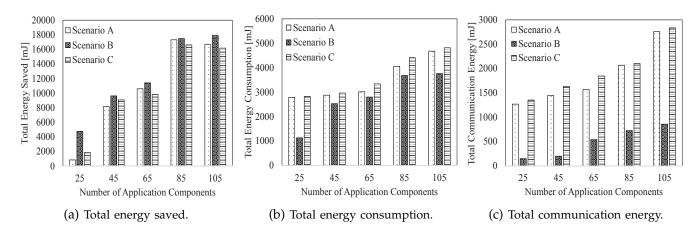
Fig. 17: Total energy versus the number of application components with Fan-in/Fan-out CDGs (maximum in-degree is 3 and maximum out-degree is 2), presented in Scenarios A, B, and C.
