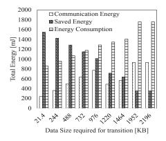
Fig. 11: Total energy versus required data size for transition of components while T=3 s,  $R_u=0.8$  Mbps and  $R_d=1.76$  Mbps using the applied CDG.
