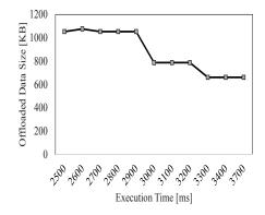
Fig. 10: Allocated data size for cloud offloading in correspondence with execution time (T) while  $R_u$ =0.8 Mbps and  $R_d$ =1.76 Mbps.
