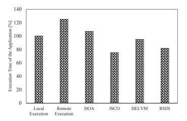
Fig. 4: Total execution time of the application for the proposed and classical schemes, normalized to the execution time by local execution (using the face recognition application in [30]).
