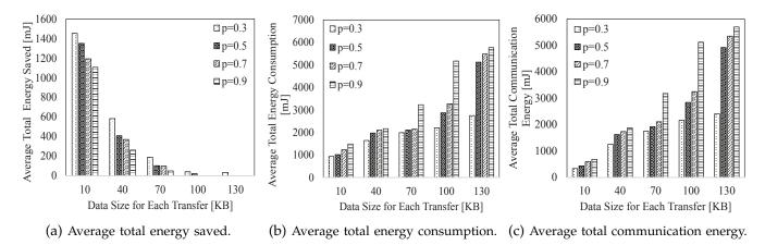
Fig. 12: Average total energy versus required data size for transferring each component in the apps with Layer-by-Layer CDG (s = 5) and 14 components while T=3 s,  $P_{Tx}=257.83$  mW,  $P_{Rx}=123.74$  mW.
