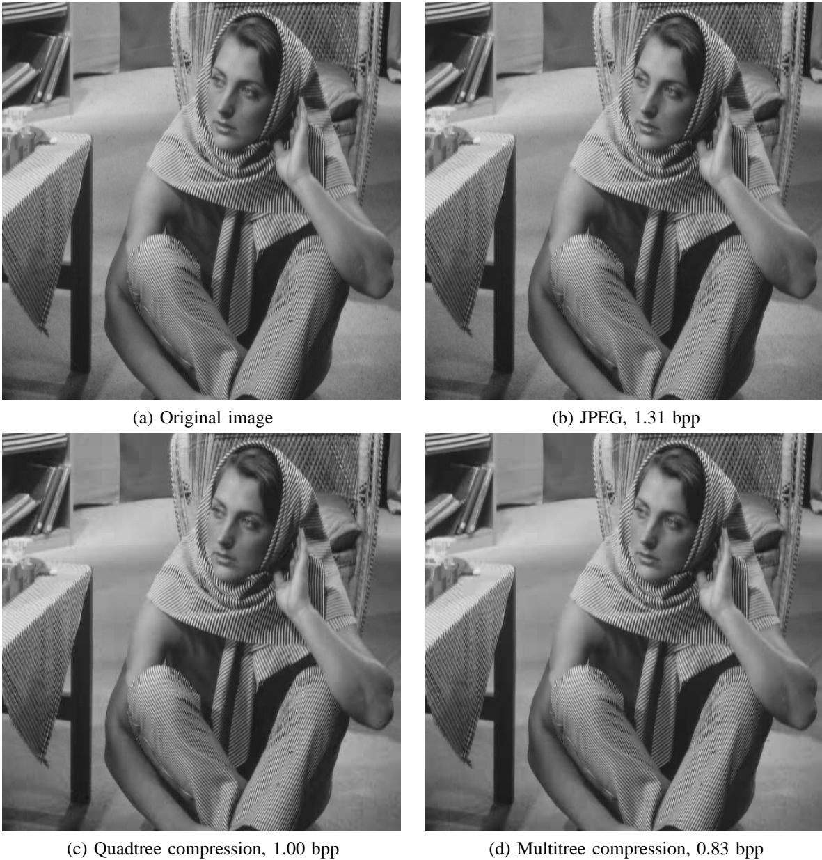
Fig. 10. Compression results for the “barbara” image at PSNR = 36.4 dB: (a) original image, (b) JPEG (rate = 1.31 bits per pixel), (c) quadtree compression (rate = 1.00 bits per pixel), and (d) multitree compression (rate = 0.83 bits per pixel).
