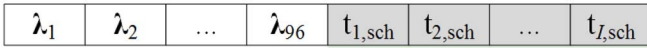
Fig. 3. Chromosome structure for the GA. The genes \lambda_1, \dots, \lambda_{96} represent the CIP vector, one element for each 15-min interval in the 24-h period. The genes t_{1,sch}, \dots, t_{I,sch} represent the schedule for the I customer loads that are schedulable.
