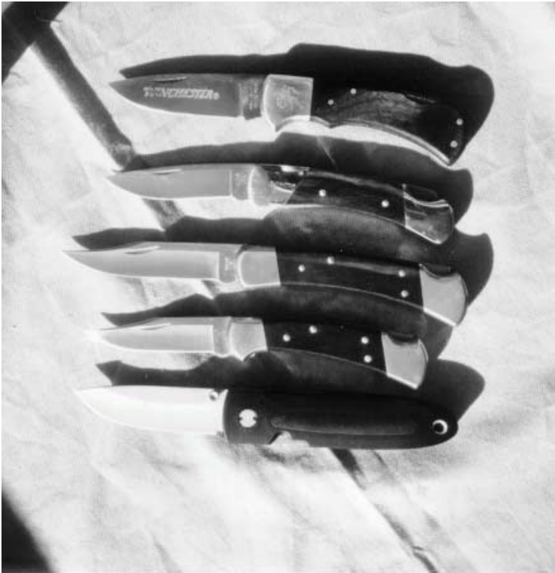
Abbildung 3.15: Klappmesser (Buck). Von oben: Winchester P107, Klinge: 440, Backen: Neusilber, Griff: Pakkaholz. Buck 500 Duke, Klinge: 425M, Backen: Edelstahl, Griff: Holz. Buck 110 Folding Hunter, Klinge: 425M, Backen: Messing, Griff: Palisander. Buck 112 Folding Ranger, Klinge: 425M, Backen: Messing, Griff: Palisander. Buck 180-D1 CrossLock Hunter, Klinge: 425M, Griff: Elastomer. Sammlung: Lüddecke
