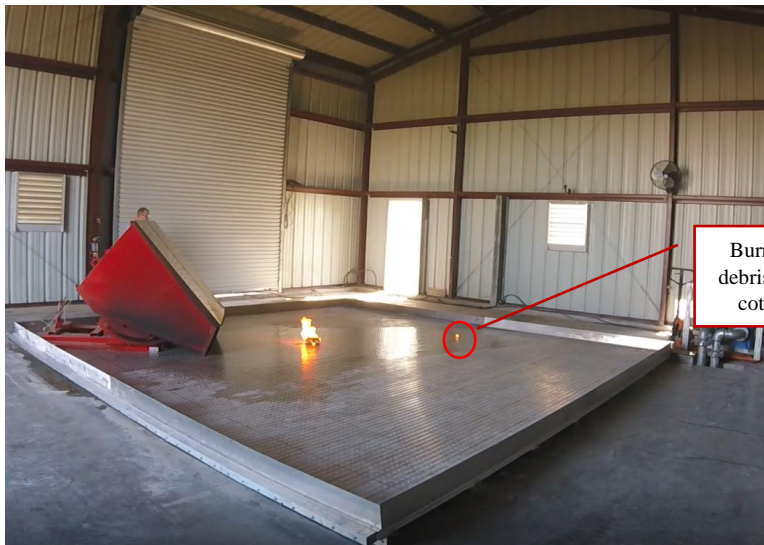
1:30 – Liquid fuel fire fully extinguished. Only fire fueled by igniter and associated debris remains on floor assembly.
