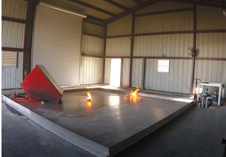
1:06 – Igniter continues to burn. Residual fuel flares up occasionally near the trench drain.
