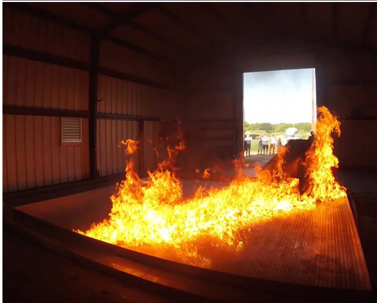
0:11 – At peak intensity, fire covers entire spill area (11 m 2 , 118 ft 2 ) and reaches a maximum flame height of 4.6 meters (15 feet).
