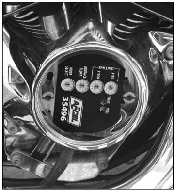
Figure 3A - Finished Big-Twin® Installation
