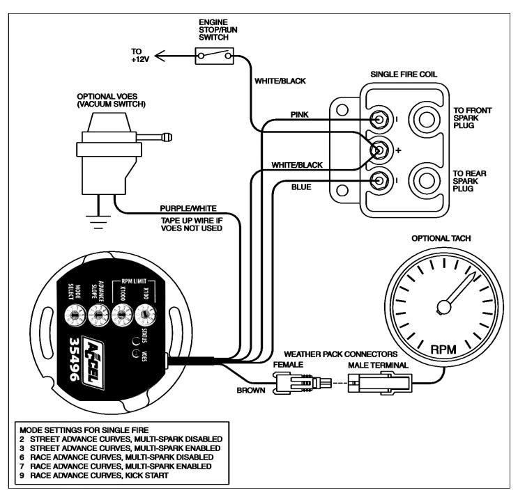
Figure 5 - Single Fire Wiring Diagram
