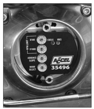
Figure 3B - Finished Sportster® Installation
