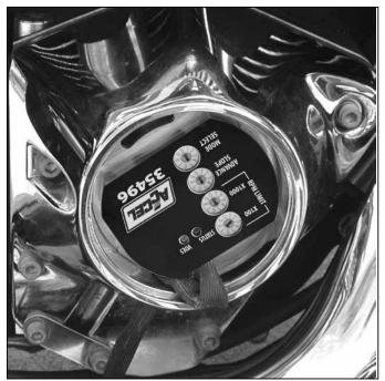
Figure 2 - Installing Unit (Note Orientation)
