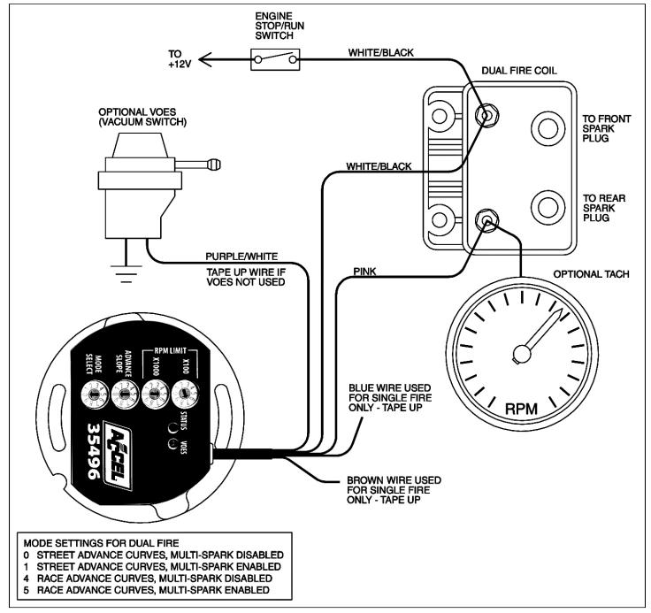
Figure 4 - Dual Fire Wiring Diagram
