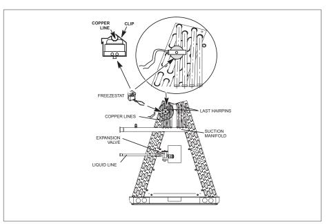
Figure 6. Typical Freezestat Installation - Indoor Coil
