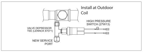
Figure 5. Tee and Vapor Line High Pressure Switch
