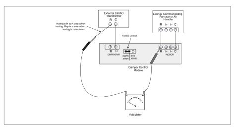
Figure 3. Confirming Correct Transformer Phasing
