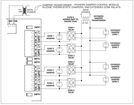
Figure 4. Damper and Extended Damper Wiring Diagram
