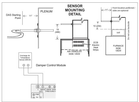
Figure 2. Discharge Air Temperature Sensor Installation (Typical Up-Flow Furnace)
