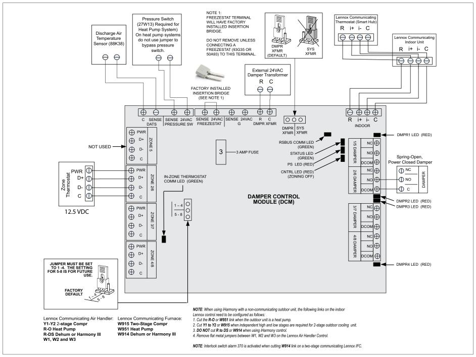
Figure 7. Damper Control Jumpers LEDs and Connections
