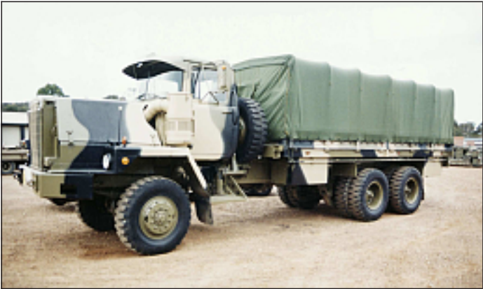
Truck, Cargo, Heavy, MC3 with standard cargo/troop carrying body and tarpaulin (Ron Fry) 1124780
