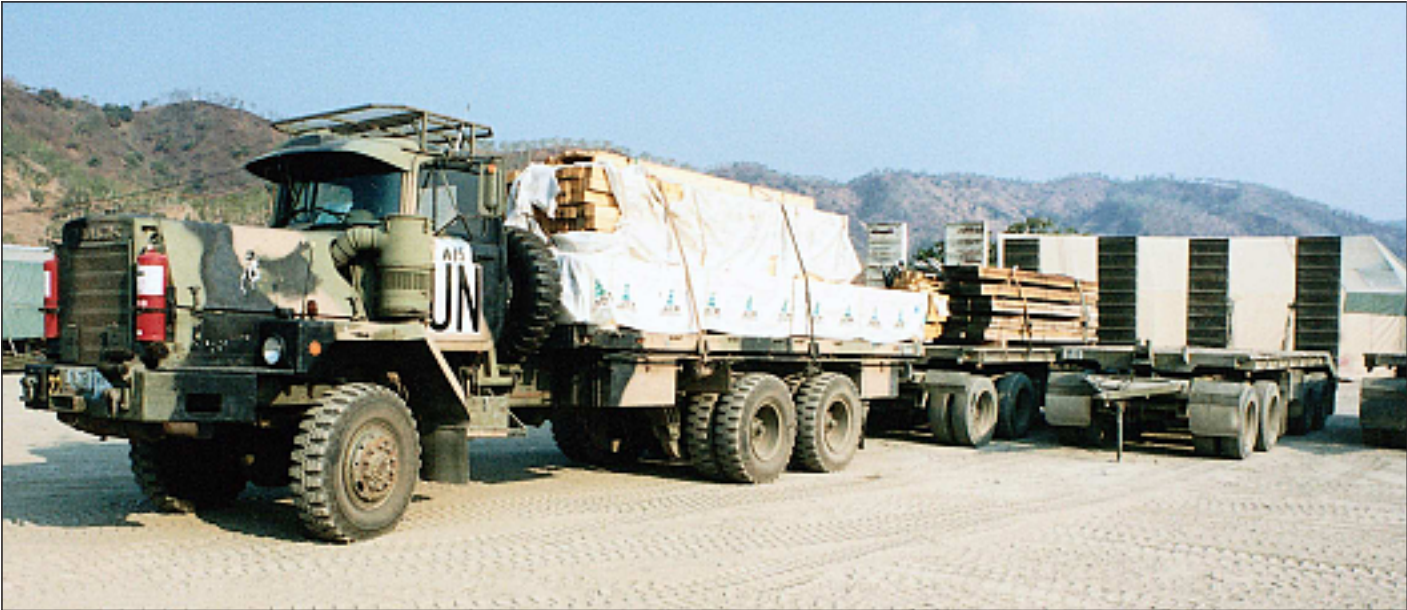
Truck, Cargo, Heavy, MC3 with winch, laden with timber and coupled to a 20-tonne plant trailer (Ron Fry) 0121280
