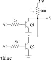
$v_1 = 0.2 \text{ V} \rightarrow i_{B1} = i_{C1} = 0, \quad v_{BE1} = 0.2 \text{ V}, \quad v_{CE1} \text{ can be anything}$
