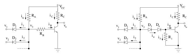
**Example:** Verify that the DTL circuit above (with  $R_A = 5 \text{ k}\Omega$ ,  $R_C = 1 \text{ k}\Omega$ ,  $R_1 = 5 \text{ k}\Omega$ , and  $V_{CC} = 5 \text{ V}$ ) is a NAND gate. Assume that "low" state is 0.2 V, "high" state is 5 V, and BJT  $\beta_{min} = 40$ .
