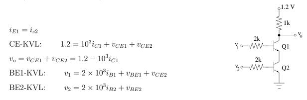
Case 1:  $v_1 = 0.4$ ,  $v_2 = 0.4$ : Assume Q2 is off  $(i_{B2} = 0, v_{BE2} < V_{D0})$ . Substituting for  $i_{B2} = 0$ in the BE2-KVL above, we get:  $v_{BE2} = v_2 = 0.4 < 0.7 = V_{D0}$ . Thus, Q2 is off and  $i_{C2} = 0$ . Since  $i_{E1} = i_{C2} = 0$  and  $i_{E1} = i_{C1} + i_{B1} = 0$ , we should have  $i_{C1} = 0$  (because  $i_{C1} \ge 0$  and  $i_{B1} \ge 0$ ). Then, from CE-KVL above:
