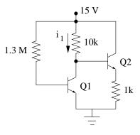
Assume Q1 is ON,  $V_{BE1} = 0.7$  V and  $i_{B1} > 0$ . BE1-KVL gives:
