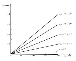
The slope of  $i_D$  versus  $v_{DS}$  line is the conductance of the channel. For  $v_{GS} \leq V_t$  no channel exists (zero conductance). As value of  $v_{GS} - V_t$  increases, channel becomes wider and its conductivity increases (because its *n*-type charge concentration increases). Therefore, the channel conductance (slope of  $i_D$  versus  $v_{DS}$  line) increases with any increase in  $v_{GS} - V_t$  as is shown above.
