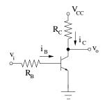
To find the transfer function of this gate, we need to find  $v_o$  for a range of  $v_i$  values. This plot will also help identify the values of  $v_{IL}$  and  $v_{IH}$ .
