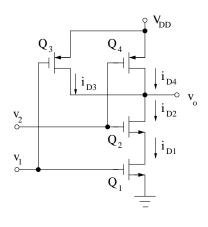
above, we have  $v_o = v_{DS1} + v_{DS2} = V_{DD}$ . This gives  $v_{DS1} = V_{DD}$  and  $v_{GS2} = v_2 - v_{DS1} = 0 - V_{DD} = -V_{DD} < \bar{V}_t$ , a contradiction of of Q2 being ON. Therefore, Q2 should be OFF.
