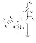
$$i_{1} = \frac{v_{BE}}{R_{1}} \qquad i_{2} = i_{B} + i_{1} \approx i_{1} = \frac{v_{BE}}{R_{1}}$$
