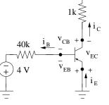
So BJT is not in cut off and BJT is ON. Set  $v_{EB} = 0.7 V$  and use BE-KVL to find  $i_B$ .
