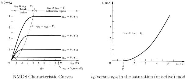
$i_D$  versus  $v_{GS}$  in the saturation (or active) mode
