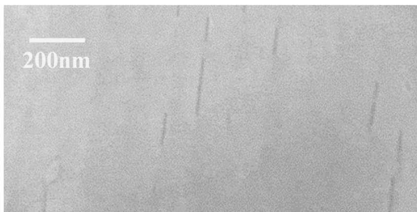
Figure 3.4 SEM image of GaP grown on silicon after proper growth temperature optimization.
