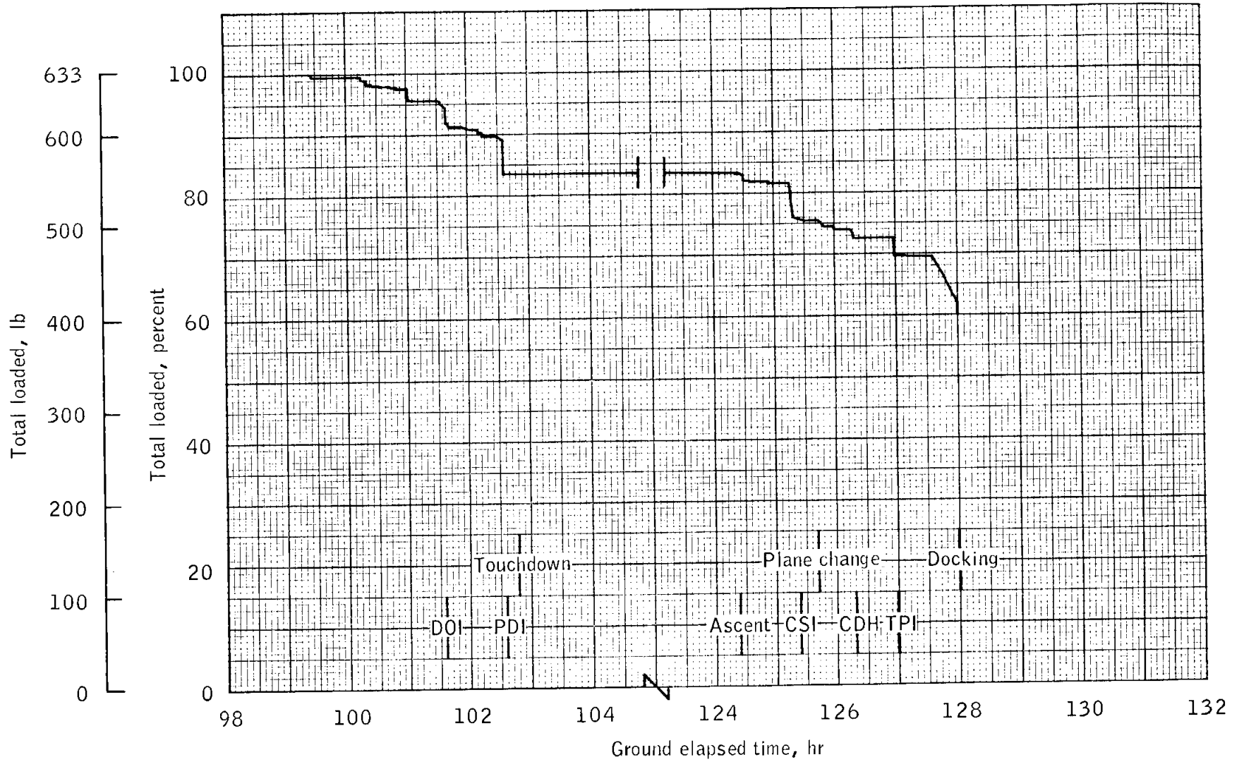
Figure 5-6.- LM RCS propellant profile.
