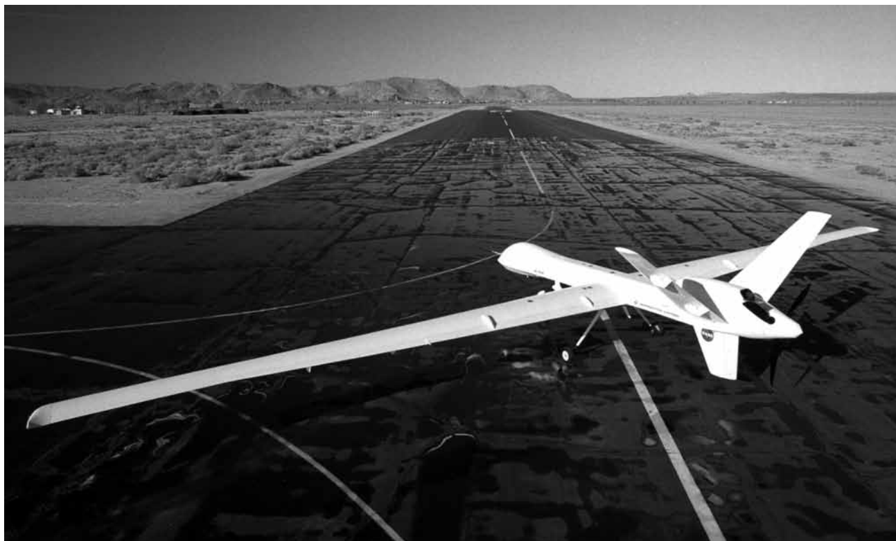
The Altair operated by NASA had an 86-foot wingspan to optimize the aircraft for high-altitude flight. The Altair was designed to carry a 3,000-pound payload to 52,000 feet.
