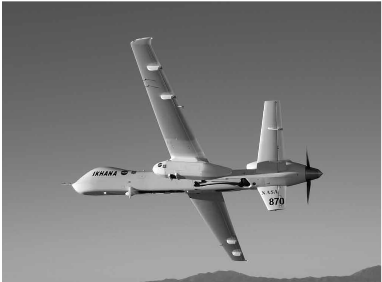
Carrying its sensor pod, the Ikhana banks away during a checkout flight in the Western States Fire Mission.
