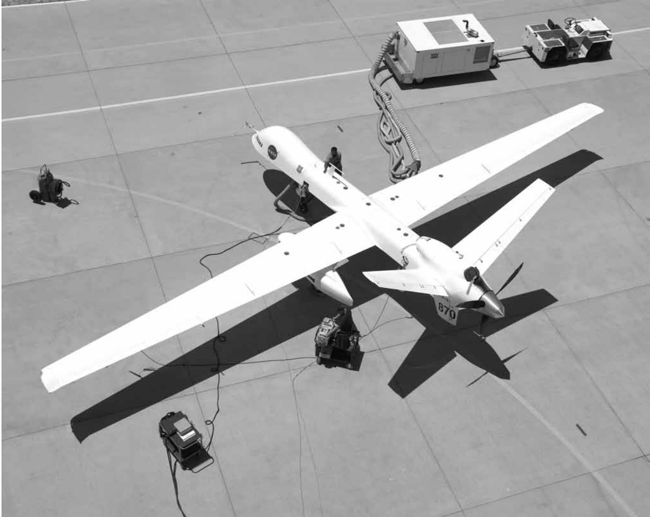
Ground crewmen prepare the Ikhana for flight. The vehicle is a civilian version of the MQ-9, modified and instrumented for use in a variety of civil research roles.
