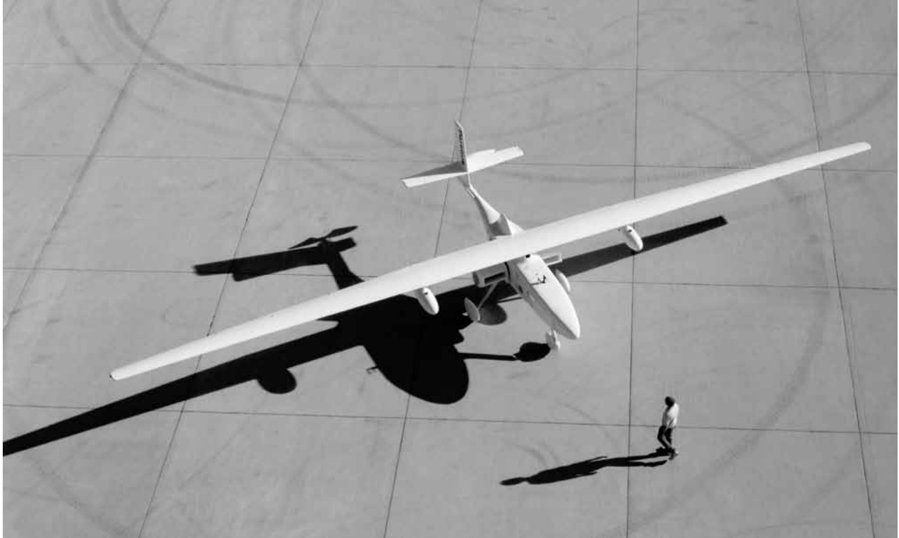
As with the Perseus-A, the Perseus-B was flown remotely by a pilot from a mobile flight control station on the ground. A Global Positioning System unit provided navigation data for continuous and precise location during flight. The ground control station featured dual independent consoles for aircraft control and systems monitoring. NASA
