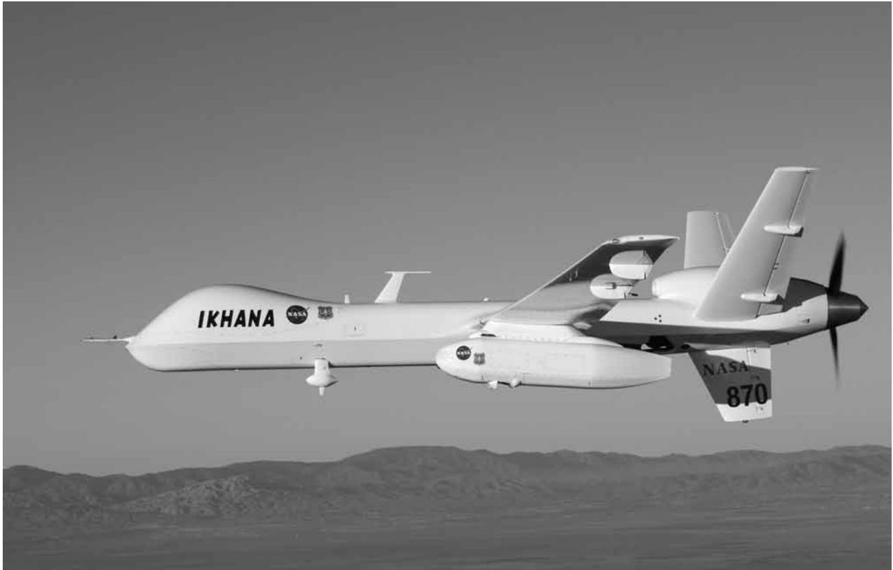
With its sensor pod under the left wing, NASA's remotely piloted Ikhana unmanned aircraft cruises over California during the Western States Fire Mission.
