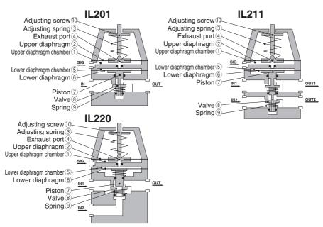
The signal air pressure enters the upper diaphragm chamber ① to generate a force. When this force is larger than the force generated by compressing the adjusting spring ③, the upper diaphragm ② is pushed up, the exhaust port ④ is closed, and the signal air pressure enters the lower diaphragm chamber ⑤ and acts the lower diaphragm ⑥. This pushes down the piston ⑦ to open the valve.
