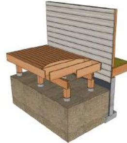
..... Open Deck - Independent Structure (Post Support) .....
