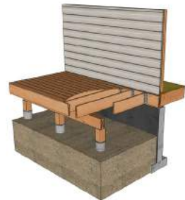
..... Open Deck - Ledger Attachment .....
