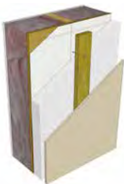
Screws through rigid exterior insulation
