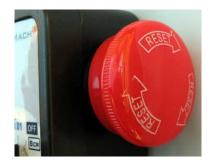
When the button is pressed and locked, "E-STOP" on LCD flashes at 1/2 second rate.
