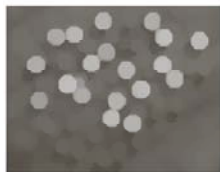
Opening by SE of radius 20. Small dowels disappeared.
