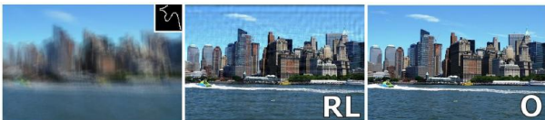
Fig. 11. From left to right: input blurred image; recovered image with Richardson-Lucy algorithm; the RL result cleaned with the mentioned algorithm.
