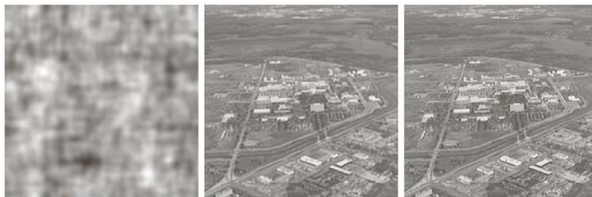
FIGURE 5.28 Comparison of inverse and Wiener filtering. (a) Result of full inverse filtering of Fig. 5.25(b). (b) Radially limited inverse filter result. (c) Wiener filter result.
