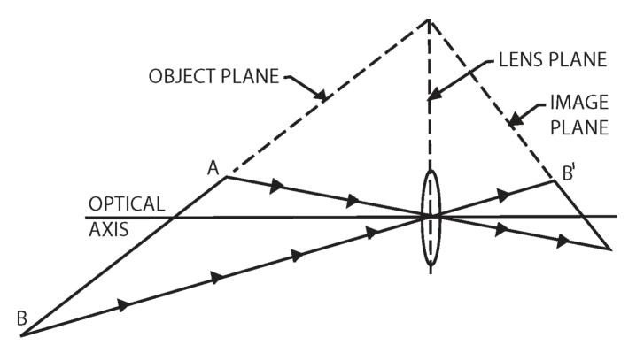
The object plane and the image plane intersect at the plane of the lens.
