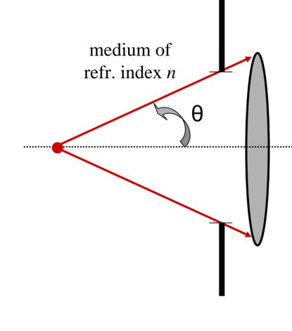
The Numerical Aperture limits the optical *energy* that can flow through the system
