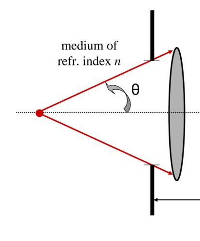
$\theta$ : half-angle subtended by the imaging system from an *axial* object
