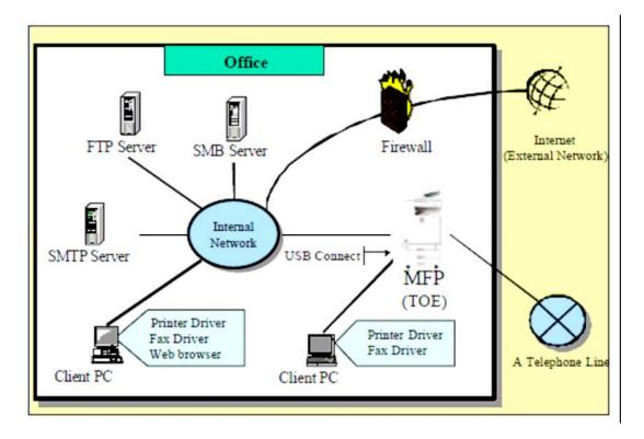
Figure 1: Environment for Usage of TOE
