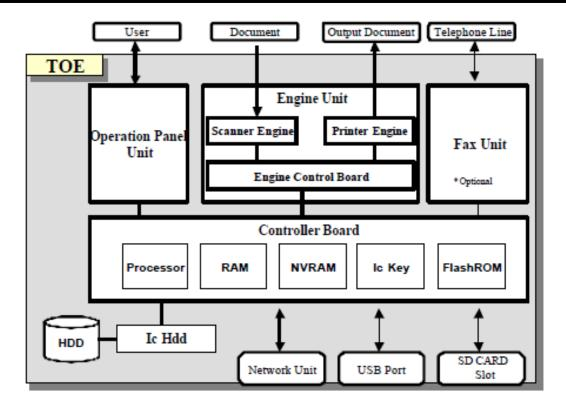
Figure 2: Hardware Configuration of TOE
