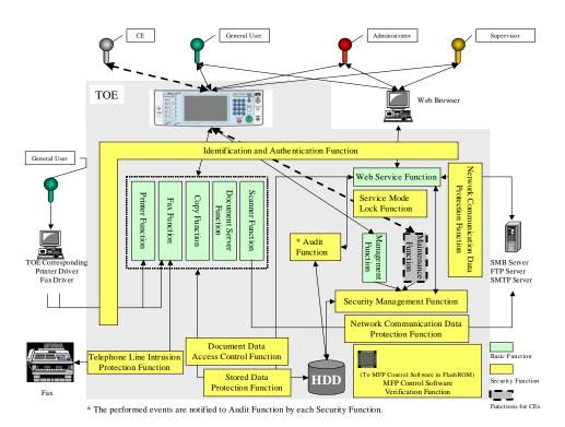
Figure 3: Logical boundary of TOE
