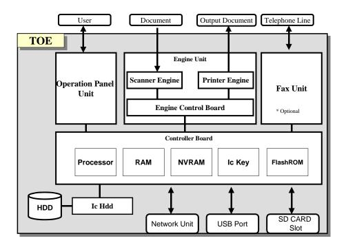
Figure 2: Hardware configuration of TOE
