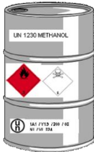
Marking and labelling UN approved drum
