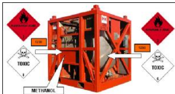
Note: hazard labels and orange signs to be affixed on four sides , proper shipping name on the two opposite sides
