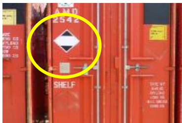
Container with ONLY dangerous goods in Limited Quantities - Limited Quantity placard on 4 SIDES
