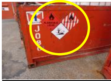
Basket loaded with dangerous goods - Placards on 4 SIDES
