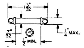
FIGURE 31. Type XI, bead-chain insulating couplings.
