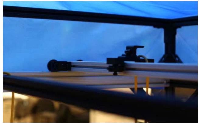
Figure 4: Horizontal sliders move in the XY plane as the user moves their arms to mimic a swimming gesture. The sliders are attached to resistance bands (in yellow), which are attached to user's arms and legs.
