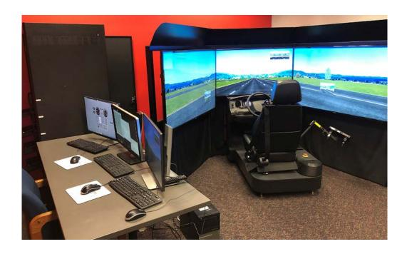
Figure 1: NJIT Driving Simulator (DS) System
