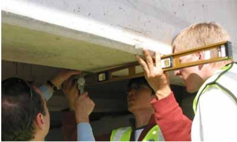
Figure 2.14: Rotation Measurement at Hutto Bridges
