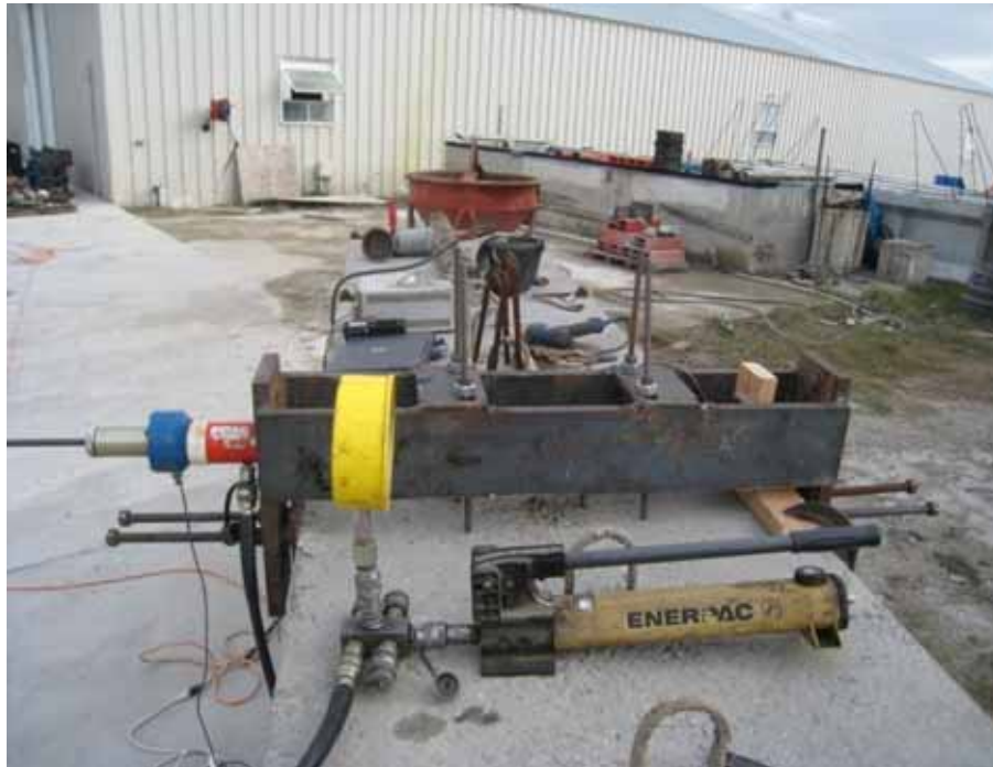
Figure 3.2: Test Setup for R-bar Testing
