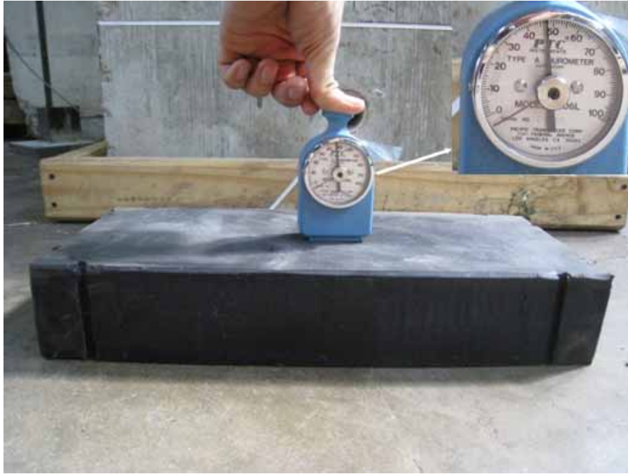
Figure 3.8: Measurement of Hardness of Bearing Pad
