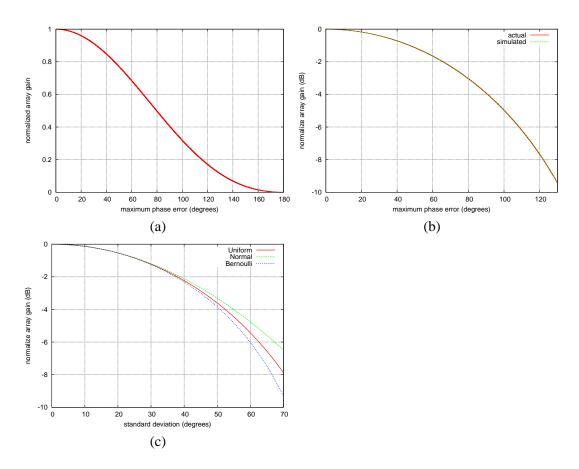
Fig. 2. (a) The normalized array gain  $\Phi(\delta_{max})$  as a function of the maximum phase error  $\delta_{max}$ . (b) The normalized array gain in dB scale,  $10 \log \Phi(\delta_{max})$ . The plot shows both the calculated gain and the simulated gain for a 10000 element array. (c) The simulated gain (dB) for a 10000 element array with different phase error distributions. For a uniform distribution, the standard deviation is  $\sigma_{\delta} = \delta_{max}/\sqrt{3}$ .
