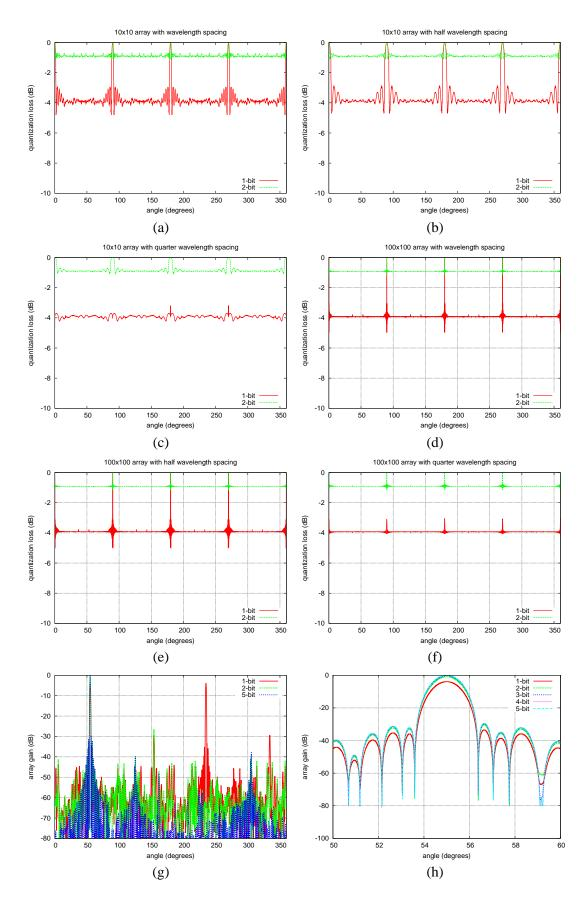
Fig. 3. (a)-(f) Array loss as a result of phase error for different size arrays. (g)-(h) 2-dimensional horizontal beampattern of a 100x100 array with  $\lambda/2$  spacing (steered towards 55 degrees) for different phase resolutions.
