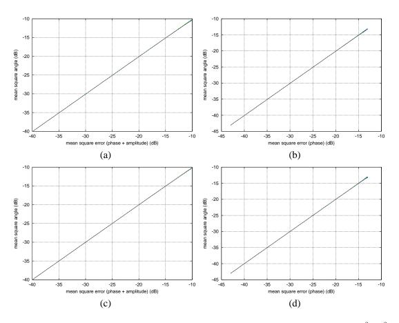
Fig. 5. Simulated relationship between phase and amplitude errors and the mean square error angle: (a),(c)  $10 \log(\sigma_{\epsilon}^2 + \sigma_{\delta}^2)$  on the x-axis,  $10 \log(\sigma_{\theta}^2)$  on the y-axis. (b),(d)  $10 \log(\sigma_{\delta}^2)$  on the x-axis,  $10 \log(\sigma_{\theta}^2)$  on the y-axis. In (a) and (b), the simulated array had 100 elements. In (c) and (d), the simulated array had 1000 elements.
