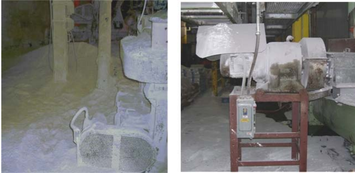
Figure 24. Deep piles of sugar accumulated on floors and equipment. Note shield installed above screw conveyor drive motor to deflect sugar dust (Imperial Sugar photos).
