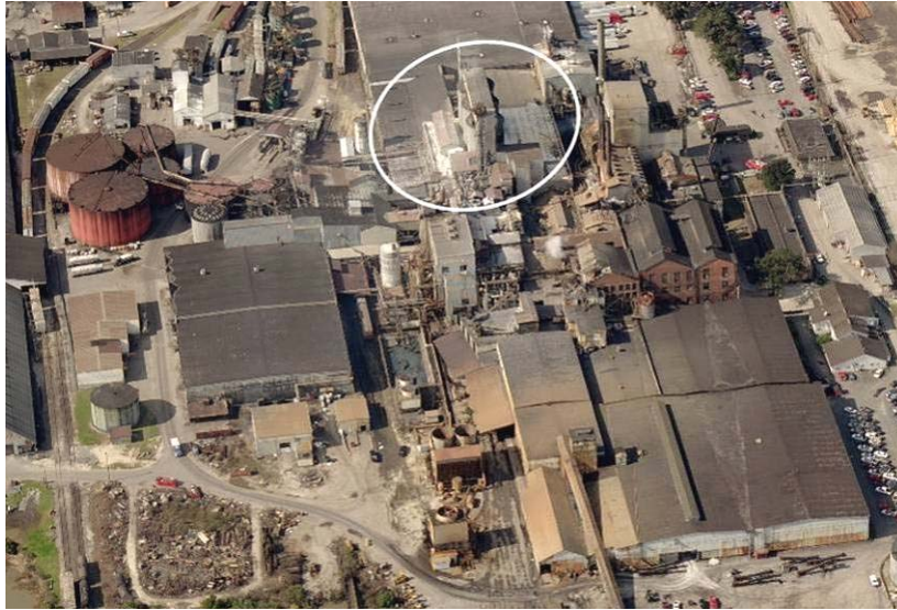
Figure 4. Imperial Sugar facility before the explosion. Granulated sugar storage silos and packing buildings are circled. Raw sugar warehouses in lower right (Chatham County, GA GIS photo)
