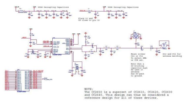
Figure 8: Reference Design Schematic
