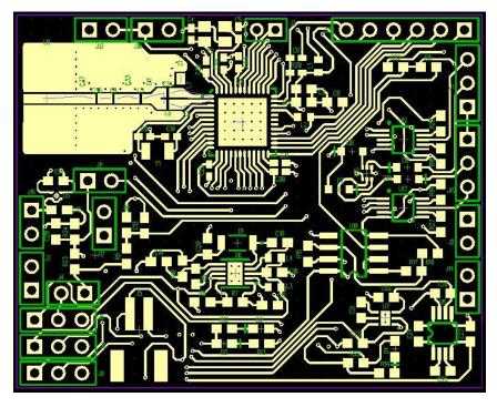
Figure 12: PCB Top Layout
