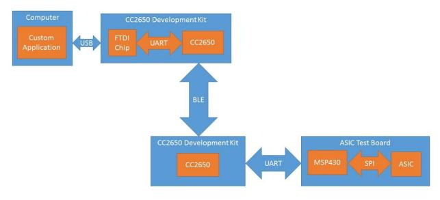
Figure 2: First System Architecture
