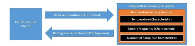
Figure 4: BLE Architecture Example – Read
