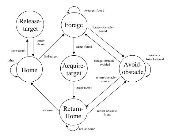
Figure 3: Finite State Acceptor Diagram
