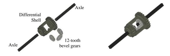
a) Pre-assembled Differential b) Assembled Differential Figure 19: LEGO Differential Gear Assembly
