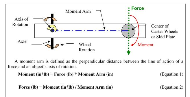
The same amount of force is required to overcome the coefficient of friction and move the robot. So, as the moment arm length increases, the moment itself must increase. In this case, the moment is the rotational movement caused by two wheels turning in opposite directions on the axle. Thus, to increase the moment, power to the two wheels turning must be increased.
