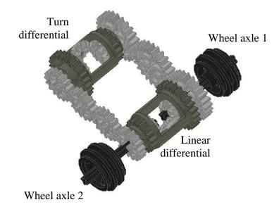
Figure 20: LEGO Dual-Differential
