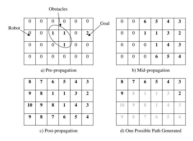
Figure 17: Wavefront Algorithm Propagation Example
