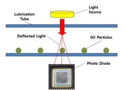
Figure 2. Oil mist lubrication sensor theory.
