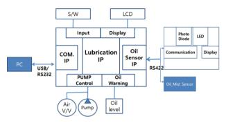
Figure 3. Block diagram of oil mist lubrication.
