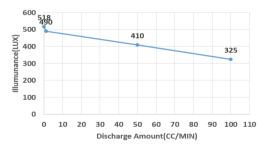
Figure 15. Measurement of colored oil mist lubrication illuminance.
