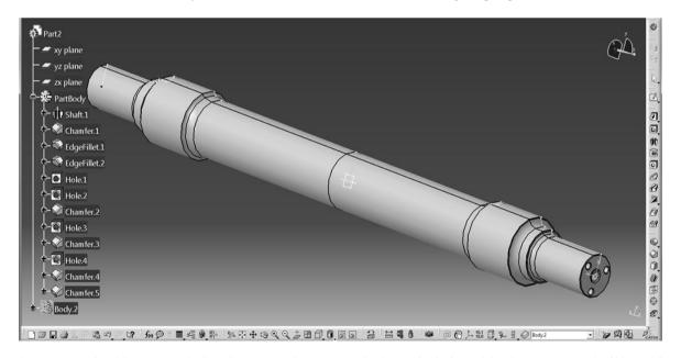
Fig. 4. process of model components in CAD/CAM system CATIA V5 Mechanical Design in the module using a tree as a work of history [6].
