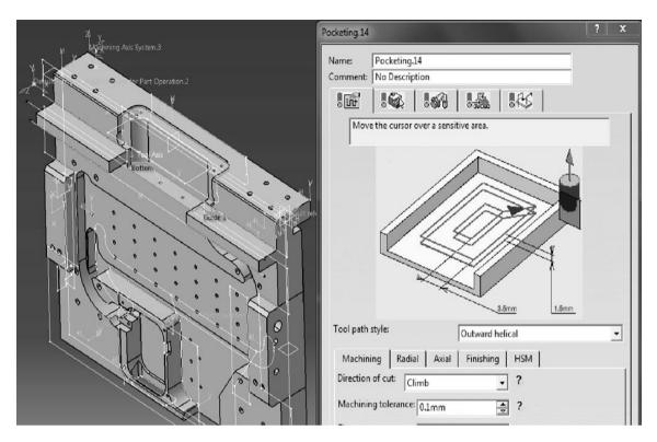
Fig. 3. strategy of prismatic milling process and dialog panel for the settings of machining simulation [11].
