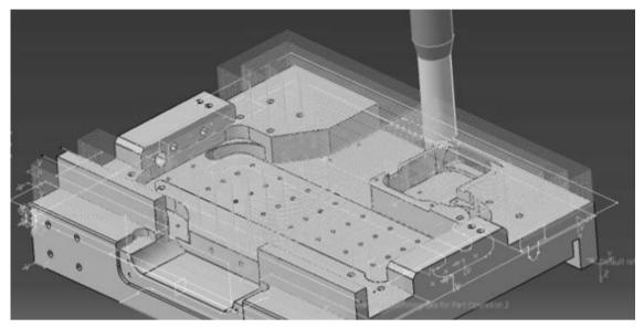
Fig. 1. prismatic milling process on selected CAD component [11].
