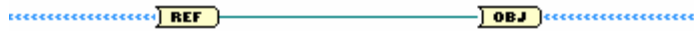
Figure 15 Creating object references with reference node and dereferencing object references with a dereference node .
