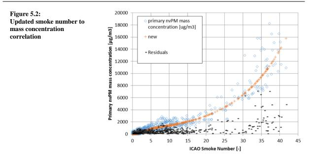
5.5.4 The new Smoke Number to nvPM mass correlation was named SCOPE11 and provides estimations of nvPM mass EIs corresponding to measured values at instrument level of an nvPM standard measurement system required for aircraft engine nvPM emission certification. An additional step was the estimation of nvPM number EIs, which is based on the nvPM mass EIs estimated from smoke number with SCOPE11 as provided by the equation below:
