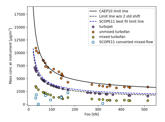
FIGURE B12: THE MASS CONCENTRATION AT 98% VISIBILITY AGAINST RATED THRUST FOR TURBOJETS IN PURPLE, UNMIXED TURBOFANS IN ORANGE AND MIXED-FLOW ENGINES IN GREEN. THE UNFILLED BLUE SQUARES REPRESENT THE MASS CONCENTRATION OF MIXED-FLOW ENGINES ESTIMATED BY CONVERTING THE MAXIMUM SN FROM THE EDB USING THE SCOPE11 METHOD.
