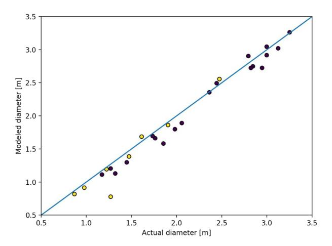
FIGURE **B10**: ACTUAL VERSUS PREDICTED DIAMETER USING THE SIMPLE GAS TURBINE MODEL. ALL ENGINES WERE MODELED AS IF THEY WERE MIXED-FLOW. ENGINES THAT ARE ACTUALLY MIXED-FLOW ARE SHOWN IN YELLOW AND THOSE THAT ARE UNMIXED ARE SHOWN IN BLUE.
