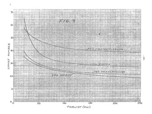
FIGURE B3: RELATIONSHIP BETWEEN SN AND RATED THRUST ADAPTED FROM MUNT (1979). THE EPA NPRM IS IDENTICAL TO THE SN LIMIT LINE, THE MIL-E-8593A IS THE CORRESPONDING MILITARY LIMIT LINE AND THE 98% AND 95% TRANSMISSION LINES ARE DERIVED BY MUNT.
