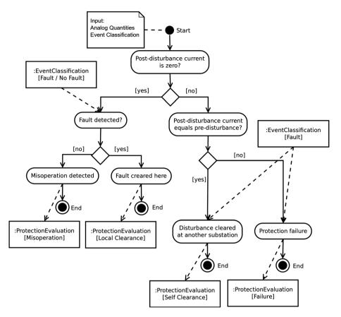
Figure 5. Protection evaluation activity diagram.
