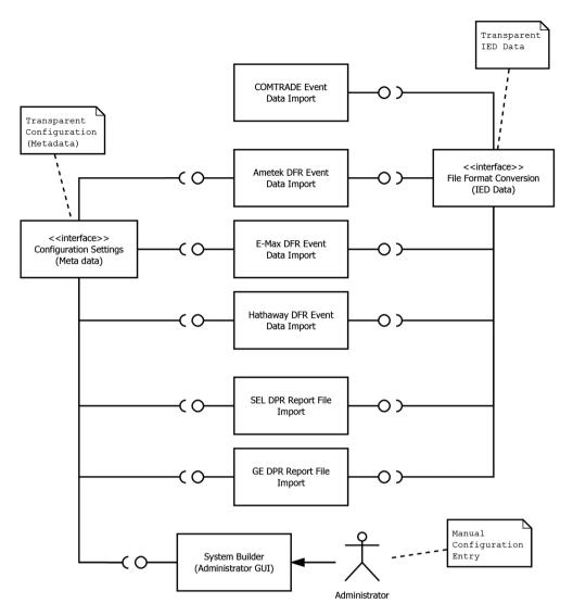
Figure 8. Implementation of the transparent data integration.
