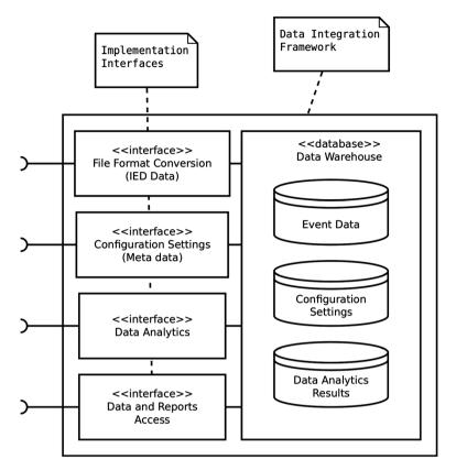
Figure 7. Implementation framework for event-triggered IED data analytics.
