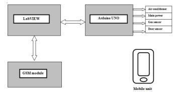
figure1(b) controlling home appliances control using labVIEW
