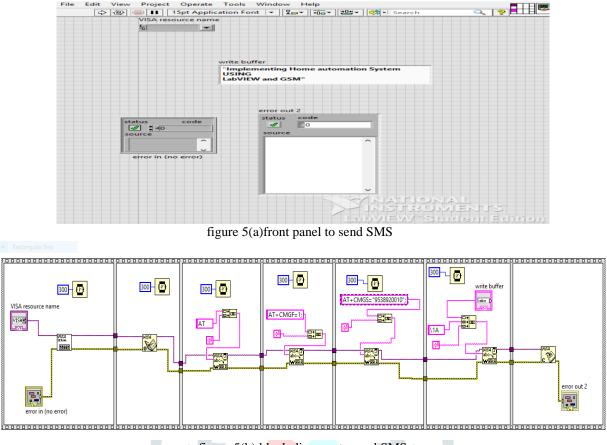
figure 5(b) block diagram to send SMS
