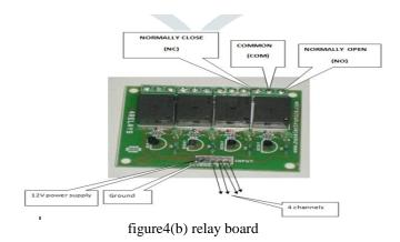
We know that most of the high end industrial application devices have relays for their effective working. Relays are simple switches which are operated both electrically and mechanically. Relays consist of an electromagnet and also a set of contacts. The switching mechanism is carried out with the help of the electromagnet. There are also other operating principles for its working. But they differ according to their applications. Most of the devices have the application of relays.
