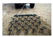
Figure 21. Chain harrow for compact tractor. (Photo from Kovar
