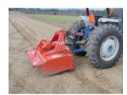
Figure 39. Heavy-duty rotary tiller on compact tractor.
