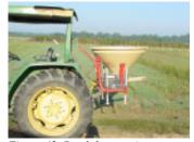
Figure 42. Pendulum-action spreader on compact tractor.
