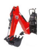
Figure 2. Backhoe for compact tractor. (Photo from BushHog)
