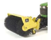
Figure 8. Rotary broom on compact tractor. (Photo from Deere and Company)
