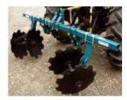
Figure 12. One-row disk bedder on compact tractor. (Photo from Buckeye Tractor Company)
