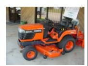
Figure 27. Mid-mount mower deck on subcompact tractor.
