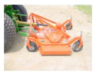
Figure 25. Heavy-duty finishing mower on compact tractor.
