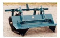
Figure 4. Bed shaper for compact tractor. (Photo from Buckeye Tractor Company)
