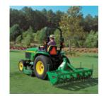
Figure 1. Turf aerator on compact tractor. (Photo from Deere and Company)
