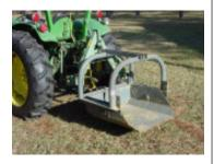
Figure 11. Dirt scoop on compact tractor.
