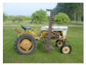
Figure 30. Sicklebar mower on small offset tractor.
