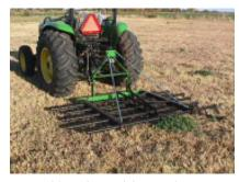
Figure 20. Spike-tooth harrow for compact tractor. (Photo from
