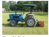
Figure 26. Flail mower on compact tractor.
