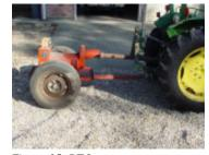
Figure 15. PTO generator on compact tractor.
