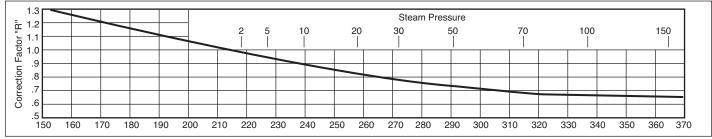
These correction factors are to be used as multipliers to correct the maximum recommended mounting heights of unit heaters when operated with steam pressures other than 2 pounds or with water at other than average temperature of 220°F.
