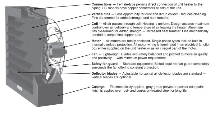
Figure 7.2 - Typical Horizontal Unit with Standard Junction Box
