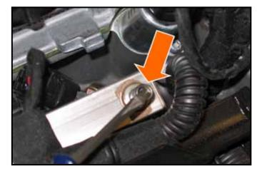
Relieve fuel system pressure by pressing on Schrader valve <arrow> and place shop cloth over valve to capture residual fuel
