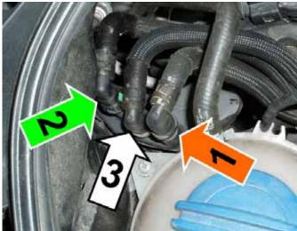
Reinstall cap for Schrader valve <arrow> located at the end of the fuel rail
