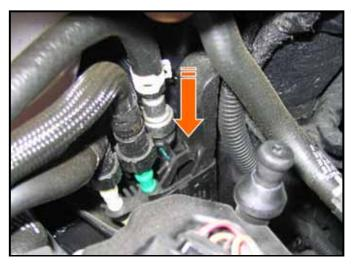
Install new fuel line (1K0 133 986 BD) line onto fuel supply line quick connect by pushing down in direction of <arrow> and ensure the quick connect is fully seated
