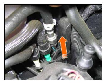
Remove fuel line quick connect from supply line by pulling back on black quick connect retainer on fuel line and pull up in direction of <arrow> on fuel line to remove it
