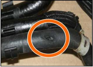
Using VAS 6340 hose clip pliers (or equivalent), maneuver and/or rotate clamp into correct position <arrow> and as shown in Section G
