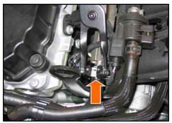
Using VAG 1921 hose clip pliers (or equivalent), remove fuel line spring clip <arrow> and fuel line from fuel rail
