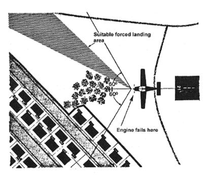
Figure 2-If engine fails at low altitude, it's reasonable to search for a suitable landing site up to 60 degrees either side of aircraft beading.
