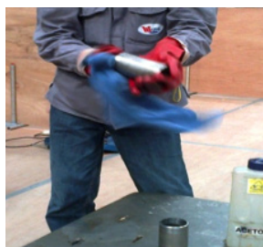
2. Clean environment The welding was carried out in a clean, air conditioned workshop with wooden floors by a single welder using new hand gloves. Both the 1 inch and 2 inch pipes were cleaned with acetone to remove all foreign particles, paints, oil and other impurities.
