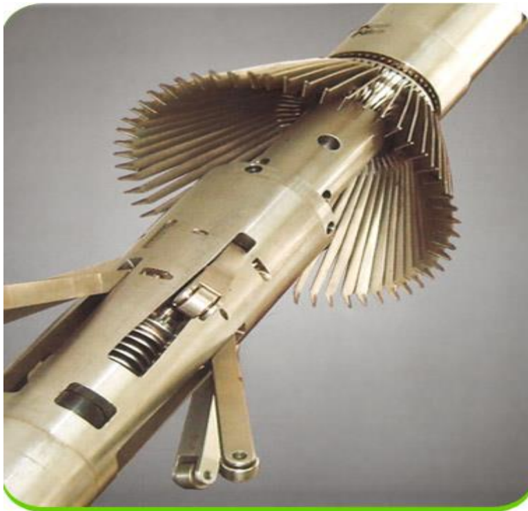
Figure 28: Caliper log tool with multiple arms
