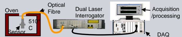
Set up for soaking tests
