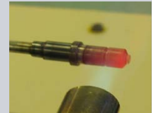
Sensor head heated to 1000°C
