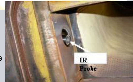
Installed probe at the combustor exit of a rig
