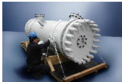
Chlorine incinerator scrubber unit, weak acid cooler
