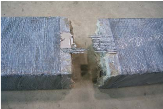
(c) CFRP rupture (beam9)
