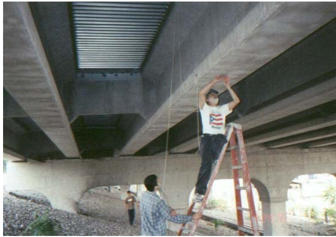
Figure 27. Installing strain gage at mid-span and monitoring responses.
