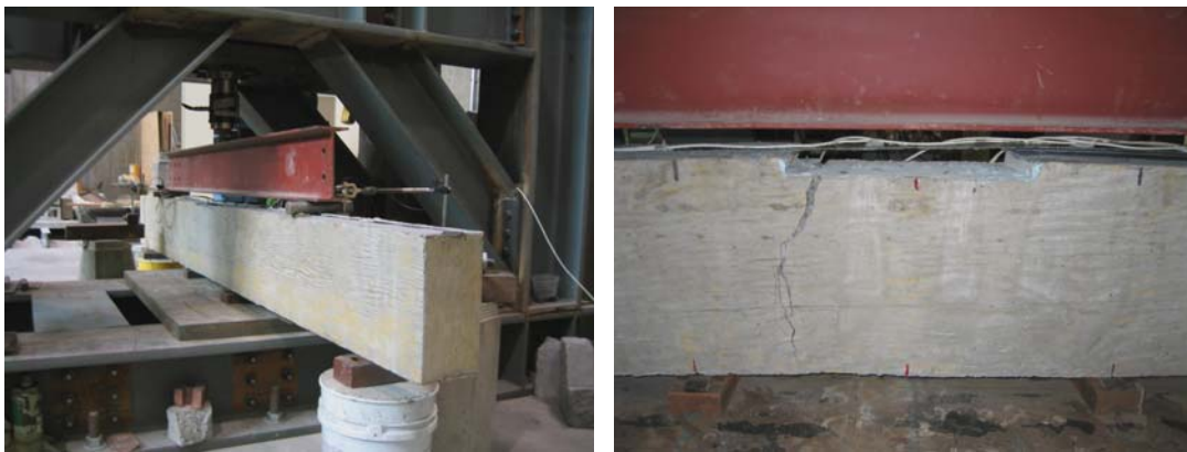
Figure 76. Test setup and failure mode of beams 3 and 4.
