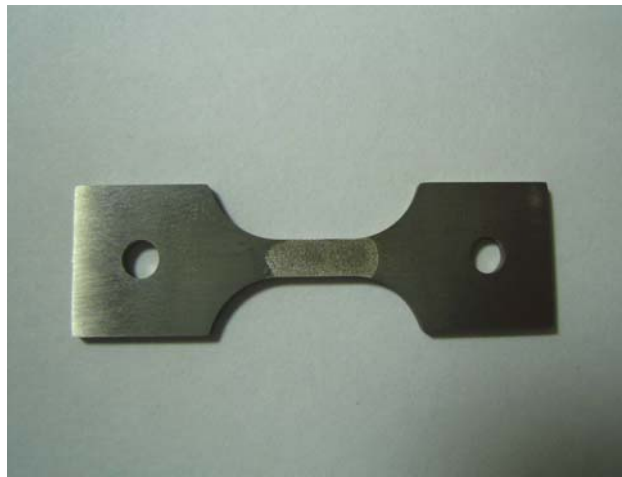
Figure 9 The fatigue specimen which is firstly machined under EDM process
