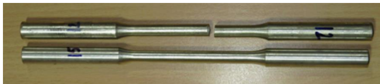
Fig. 5. Fatigue test specimen before and after the test.
